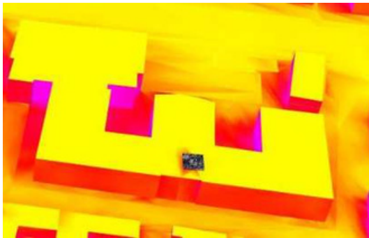
Figure 2: Snapshot from the software package PVsims for the solar irradiance incident on our school, Draschestraße
